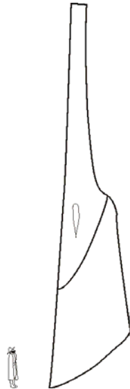
Figure 2 A quarter rudder a trading ship described in a contract written in France in 1246. The small human figure gives the scale. The rudder was 18m in length and would have weighed approximately 11,000 kg. A ship with an overall length of 54m would have required two such rudders.
